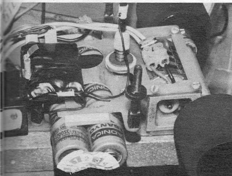
Left: competitors, Schumacher 'C'-Car fitted with a 'Quasar' speed controller produced by Star Electronics. A very neat, compact device capable of being fitted low-down on the chassis. 'C-Cars' proved to be the most popular chassis marque at the Stafford meeting closely followed by Demon then Associated.
